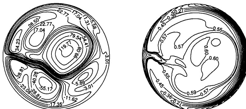
Fig. 14 Streamline and isotherm pattern for Ra_\Omega=10^7 , Ta=10^9 at \phi_g=3\pi/2
